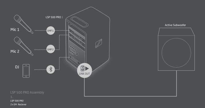
APPLICATION EXAMPLE 2: A small set-up with lots of bass here: Two wireless microphones and one Bluetooth music player are mixed on speaker 1. To add more low end, speaker 1 LINK OUT is configured to serve audio for an optional subwoofer.
