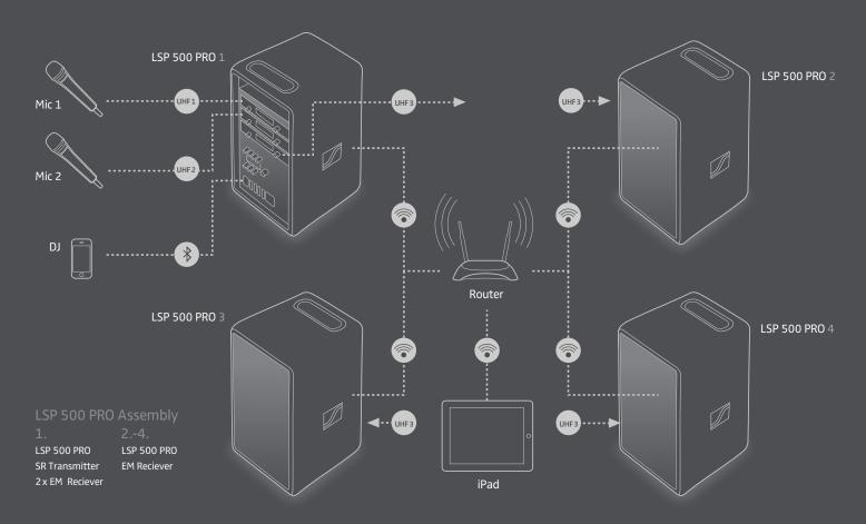
APPLICATION EXAMPLE 1: Two wireless microphone inputs plus one Bluetooth input for the DJ. All inputs are mixed on speaker 1 and wirelessly distributed to speaker 2 to 4. All LSP 500 PRO speakers within the same network – single speakers, groups or the whole system – are iPad controlled.
