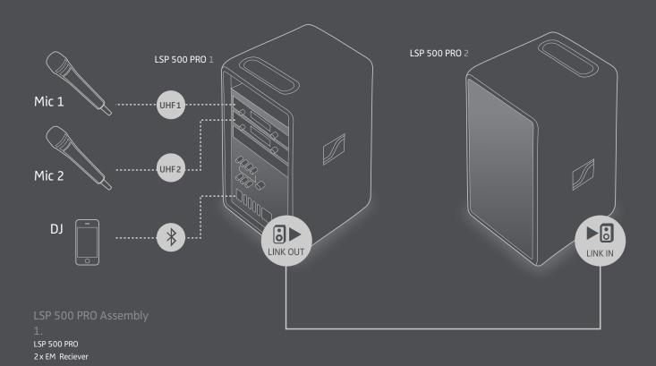
APPLICATION EXAMPLE 3: A set-up for talk and pumpin' stereo: Again, two ew 500 wireless mics and one Bluetooth music input are being mixed on speaker 1. The music is split into stereo channels – speaker 1 LINK OUT serves the right stereo channel to speaker 2 LINK IN.
