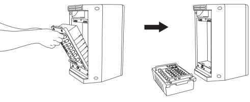
Use only the mixer's handles when removing the mixer from the speaker and when carrying the Caution mixer separate from the speaker.
